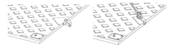
With the help of the chain sling, the panel can be moved to the desired position and installed.
