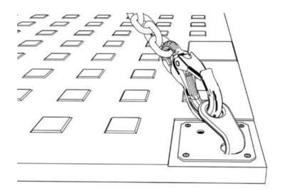
With the help of the chain sling, the panel can be moved to the desired position and installed.
