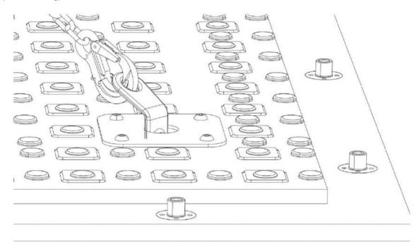
With the help of the chain sling, the panel can be moved to the desired position and installed.
