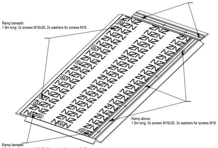
0.9m long: 2x screws M16x30, 2x washers for screws M16
