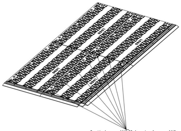
2m side: 4x screws M16x30, 4x washers for screws M16 1m side: 3x screws M16x30, 3x washers for screws M16
